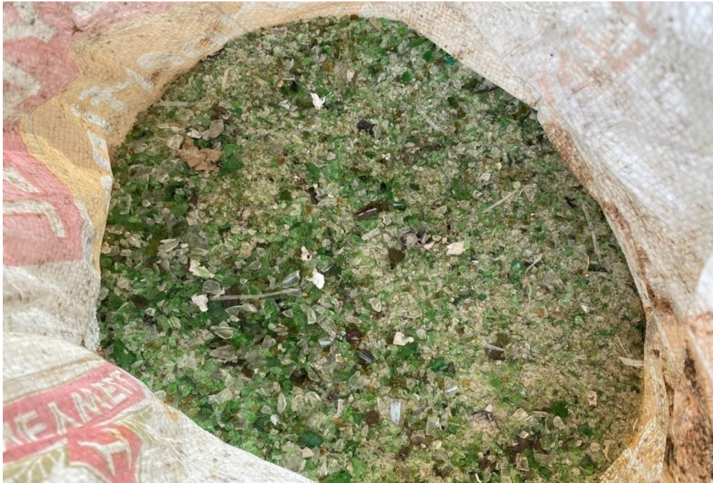
Plate 1: Grounded Broken Bottles
